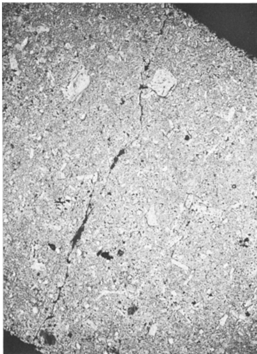
Figure 1 Polished and thermally etched specimen of beta-alumina exhibiting sodium dendrites ( \times 50 ).
